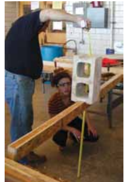
Figure 13b Students and an instructor measure the deflection
